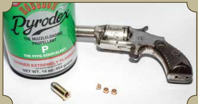
Loading for an obsolete rimfire caliber requires a little improvising with modern powder and a .22 blank for the primer.
