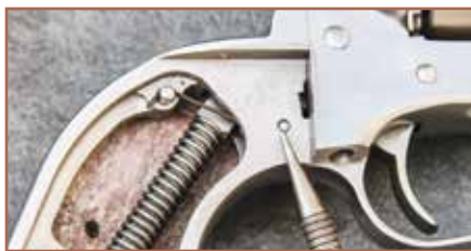
The trigger spring retaining pin — drift it out, yank the factory spring and replace with a Wolff spring. Your trigger finger will thank you.
