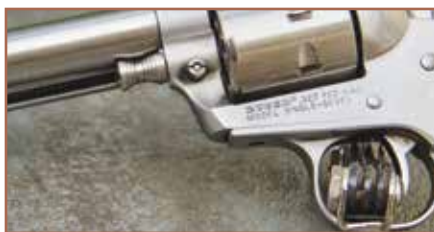
An oversized Belt Mountain base pin will tighten up your cylinder.
