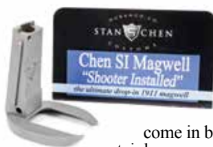
Chen's "Shooter Installed" magwell is precision CNC machined out of heat-treated 4140 carbon or 416 stainless steel billets. Photo: Roy Huntington
